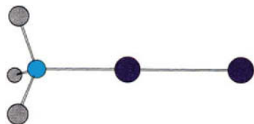
Figure 19 Crystal structure of the trimethylamine–I 2 complex. 46 The distances are N...I 2.27 Å (vdW 3.65, covalent 2.15), I–I 2.83 Å (2.70 in I 2 ).
